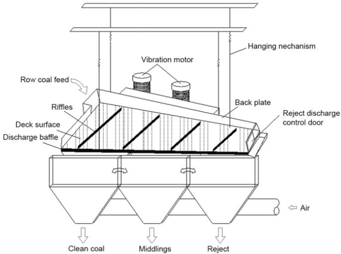
Figure 2: Structure of compound dry separator
