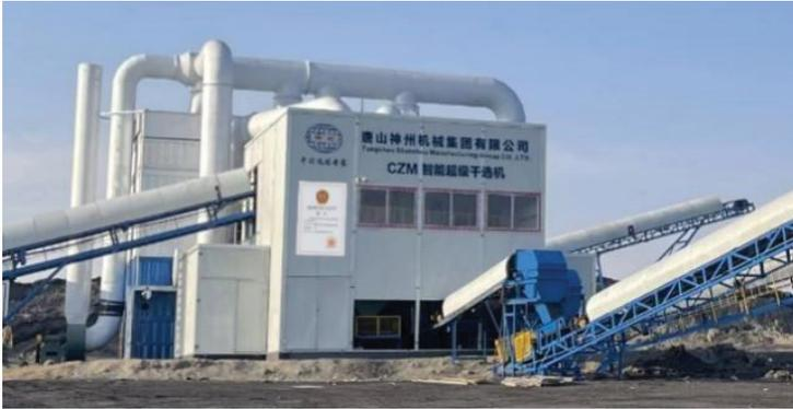
Figure 3: CZM200 Super dry separator
