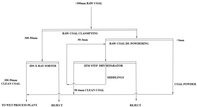
Figure 7: Coking coal deep pre-deshaling dry separation process flowsheet
