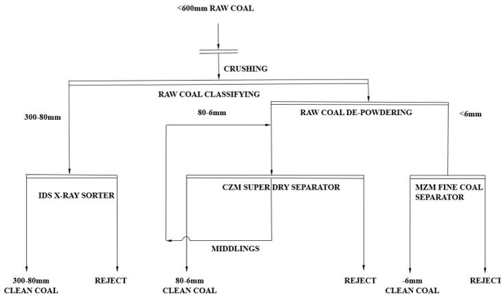
Figure 6: Thermal coal wide size range dry separation process flowsheet
